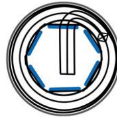
Polygonal-shaped, resilient threads
